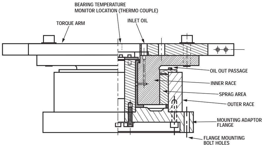
Above drawing is of typical ARD clutch and does not show all mounting adapter designs.
